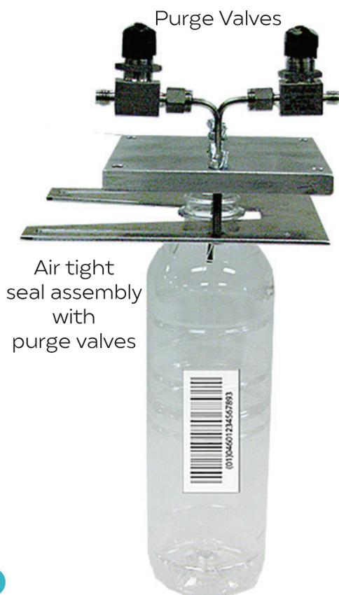
After purging the oxygen concentration within the bottle can be monitored over time
